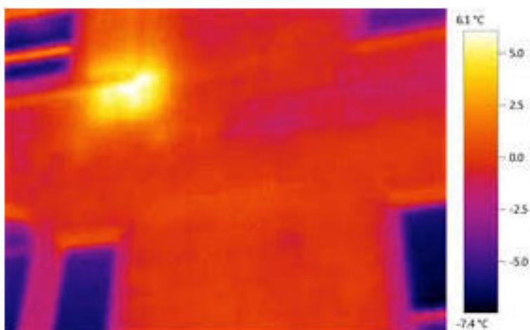
Traditionally radiators were fitted on external walls, typically under windows. Heat loss through the external wall is plain to see with the thermal image camera when looking from outside the house. It can be reduced simply by using a reflective foil behind your radiator.
