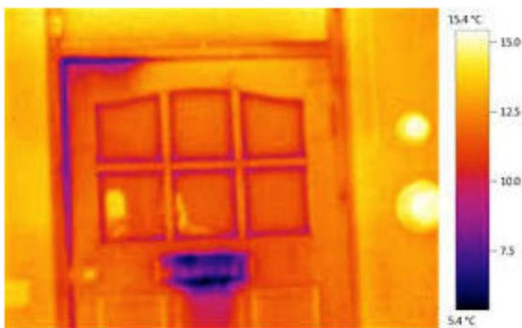
Where there is cold air showing through or around the letterbox, it can be remedied by fitting a secondary flap to the inside of the door or replacing the letterbox with a draught proof one – easily available from DIY stores.
