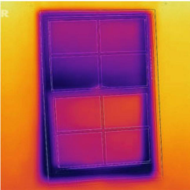
The thermal camera can show up draughts around windows. As with doors, you might want to check the blue is from the gap between the window and the frame and not just from reduced air circulation by putting a thermal finger print on one side of the gap.
