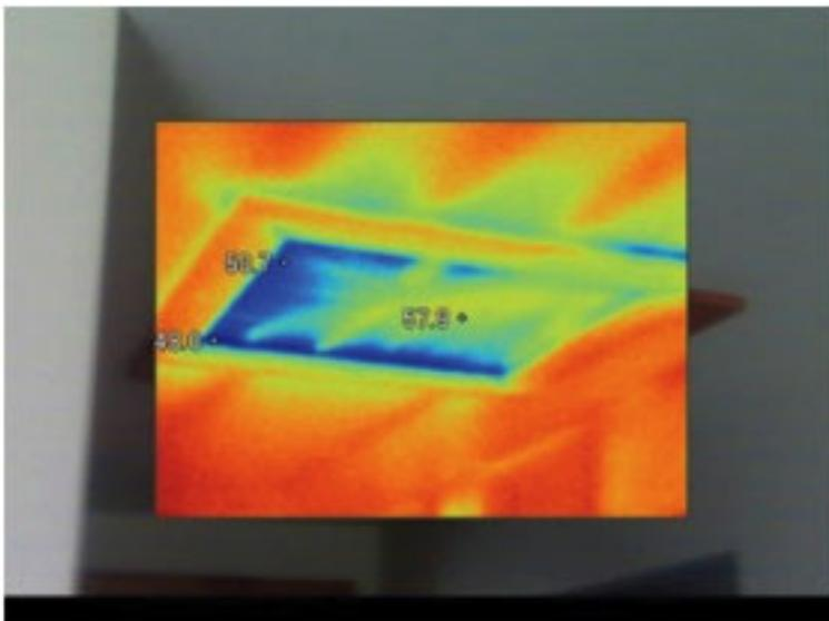
Your infra red camera will easily identify issues with attic hatches. If the loft hatch has not been insulated, it is an easy job to fit a square of board insulation to the inside of the hatch. This boarding is easily available from hardware / DIY shops – and is easily cut to size. Also consider adding draught proofing strips around the edge of the hatch.
