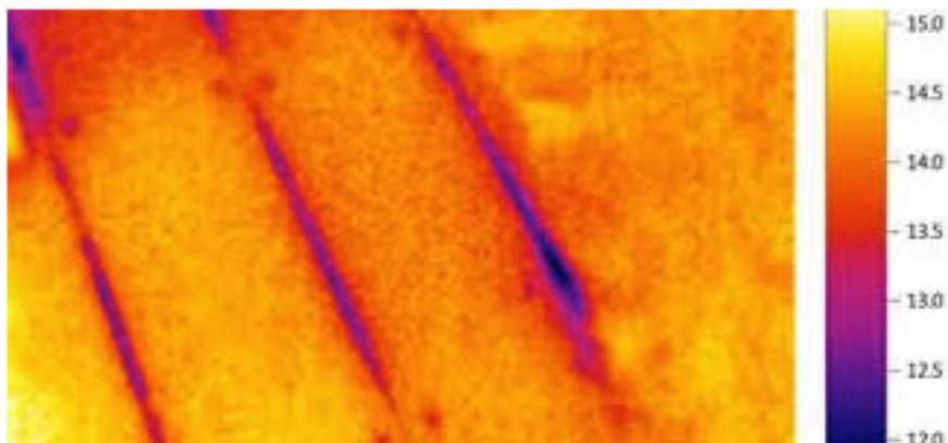
Here are areas of floor showing cold air coming through the floor boards from below. It would be worth sealing the gaps with draught excluding material such as the V shaped excluder. DraughtEx is a good solution, and specific for the job:
