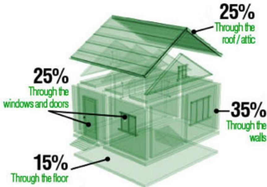
35% of heating is lost through external walls. Check the temperature of your external walls with the thermal image camera. Pointing the little circle in the middle of the screen at the wall in question and then note the temperature in degrees C in the top left hand corner. You can compare that with the temperatures of the internal walls.
