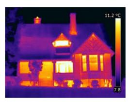
Your chimney works on the very simple principle that warm air rises and cold air sinks. This is great when you have a fire burning, enabling the smoke and fumes to escape into the atmosphere. It's not so great when you don't have a fire burning however. The same principle is still working. Your warm room air is escaping up the chimney stack, sucking in draughts. Also cold outside air can descend down the chimney.
